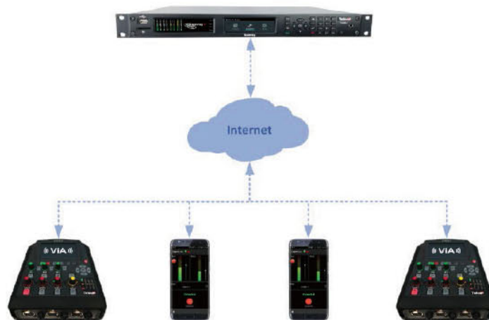
Gateway 4 Codec at a Studio Connects 4 Full-duplex Mono Remote Streams
